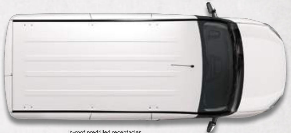
In-roof predrilled receptacles
